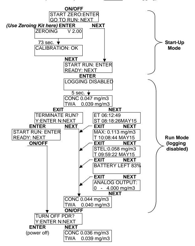
Start-Up, Set-Up and Run Mode (With Data Logging)
