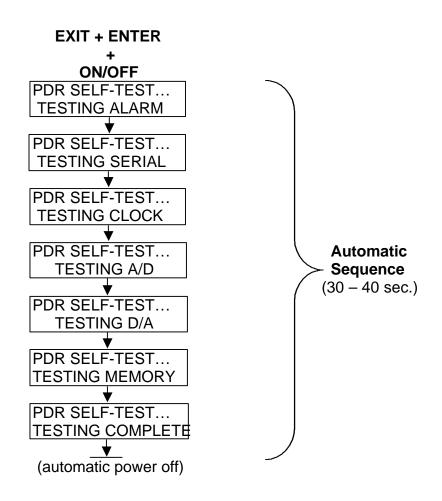
NOTE: After the preceding resetting sequence, the instrument should be zeroed, otherwise its optical background will remain unsubtracted.
